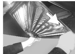
Hold the two screws on the filter mesh with both hands and pull it down to detach the two prongs inside from the filter mesh. Then pull the filter out as per the arrow direction to remove it.
